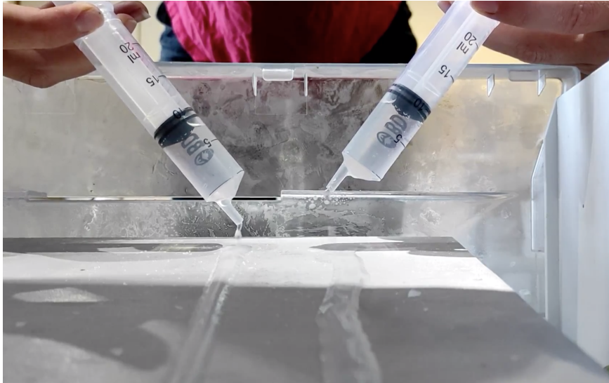
Figure 20: Syringes of fresh water (left) and salt water (right) producing trails on a cold aluminium plate in a household freezer.
