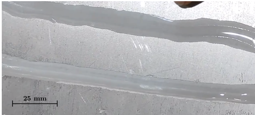
Figure 21: Resulting salt water (upper) and fresh water (lower) ice trails on the aluminium plate.
