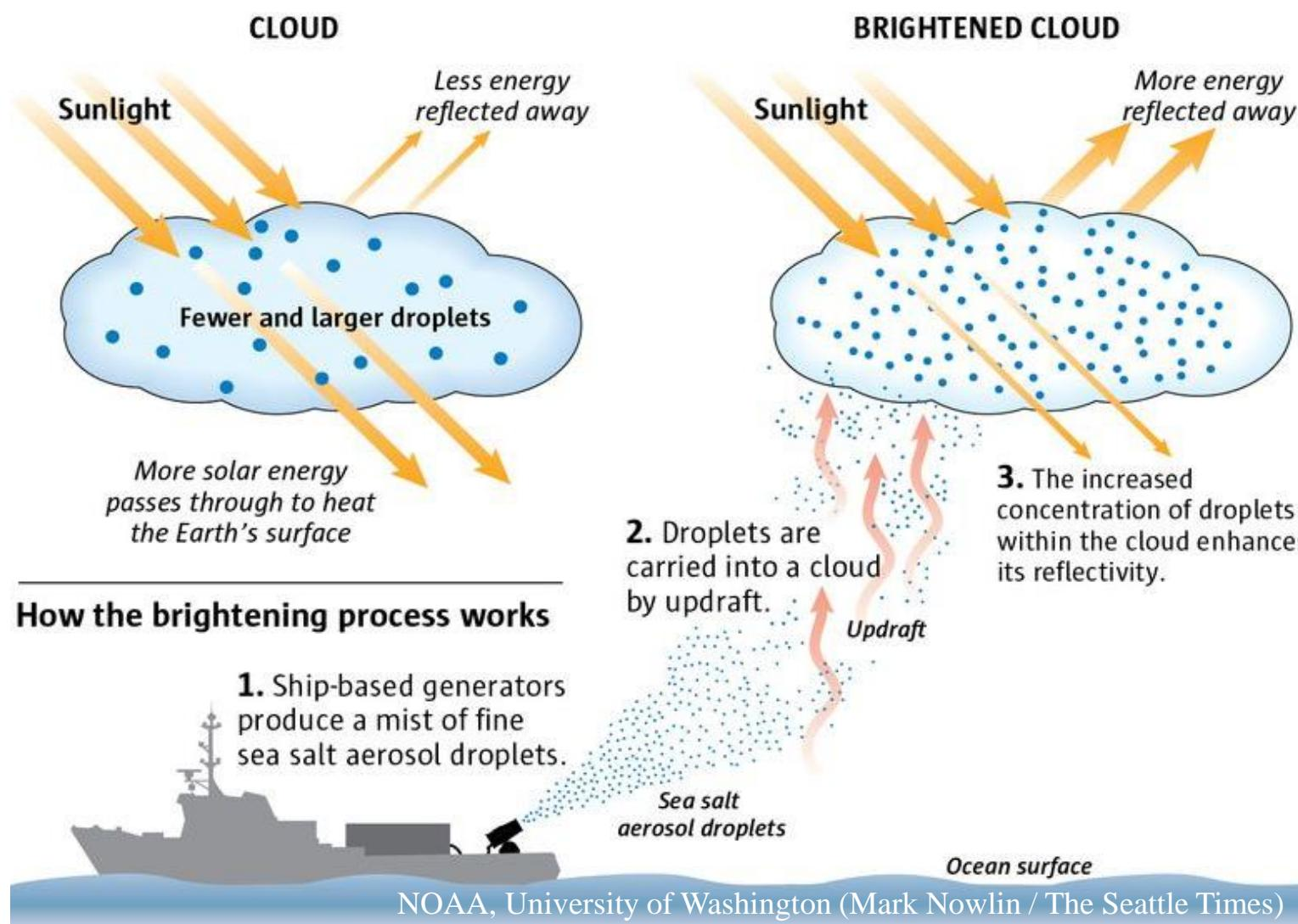
Figure 1: Marine Cloud Brightening Process [3]
