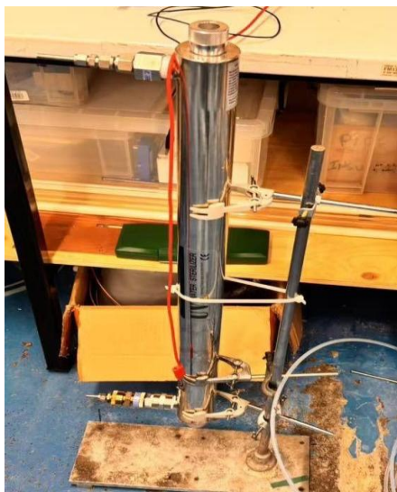
Picture: UVC light/ reaction chamber for Methane Oxidation
